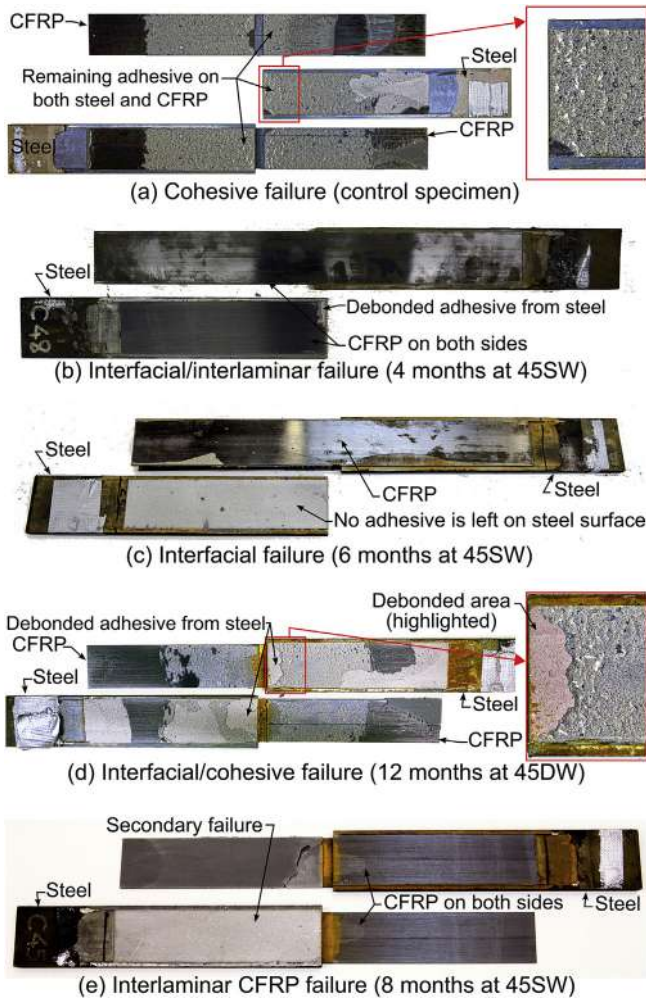
Fig. 14. Examples of fracture surfaces and failure modes of CFRP/steel specimens.
