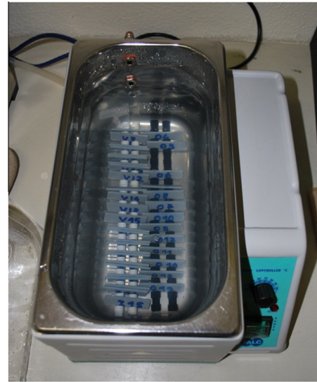
Fig. 2. The FALC WB-M15 thermostatic bath used for conditioning of the specimens.
